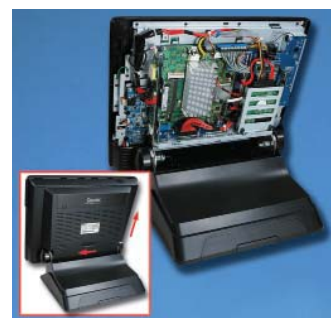
Tool-Free Access to RAM, Hard Disk Drive and Compact Flash Card Optimises Serviceability
